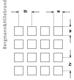
w = hole widthth = pitch horizontaltv = pitch vertical
